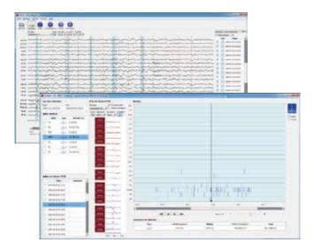
**Spike detection:** All detected spikes can be seen over a period of time over all channels on one screen. This enables you to get a quick overview on where and when spikes ocurred.
